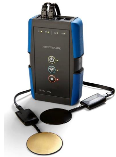
Picture 8: The CURO and sensors used to measure muscle sound. The picture is retrieved August 7, 2017 from http://www.myodynamikequine.com/amg/
